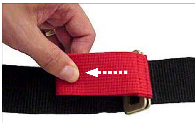
Figure 10 - Loosening the restraint
