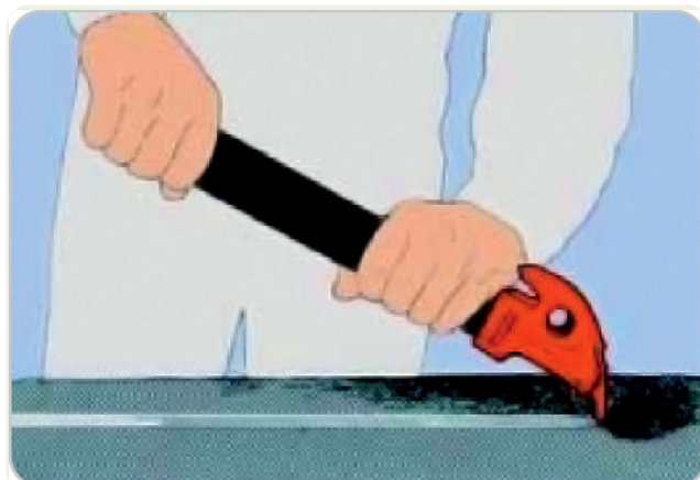
Scraping off earth, ice etc.
