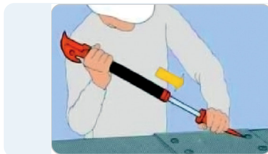
2 Cutting off rivet- and boltheads.
