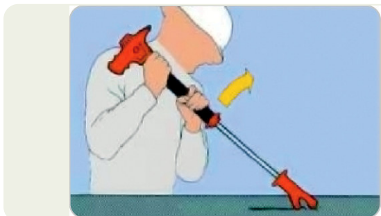
7 Long leverage in thick sheet metal (2-3 mm).
