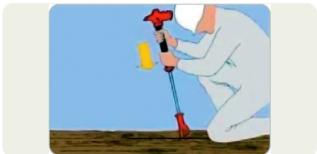
1 Pierce floor with pumping motion.
