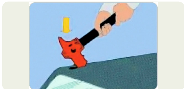
6 Car roof, etc. - slanting short hits.
