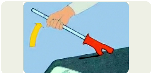
7 Rapid cutting in thin sheet metal.
