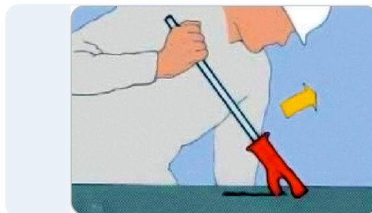
8 Only claw part in thin metal - car roofs, driver cabins etc.
