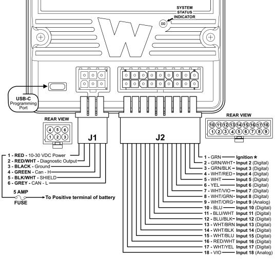
★ Connect to an ignition controlled circuit that can accommodate an additional 250 mA load.
