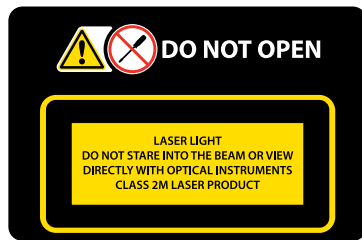
Do Not Open/Laser Notice Location: Controller Housing
