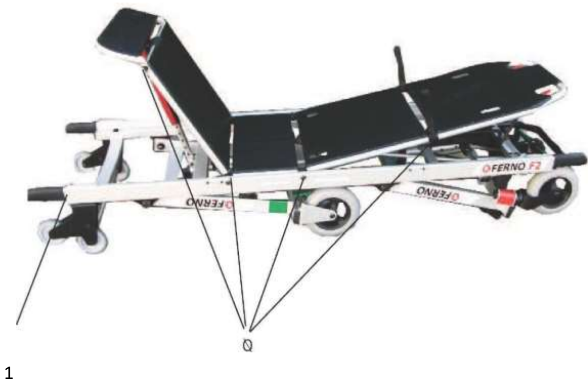
Figure 14: Lubrication of stretcher joints
