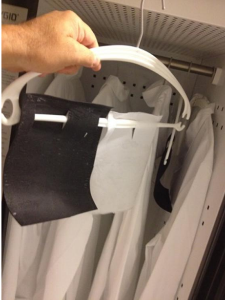
Figure 1. Test pieces ready to go to ozone treatment in Hygio.
