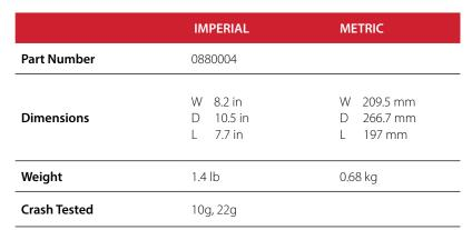
• Must be used in conjunction with Ferno D360 equipment specific mount
